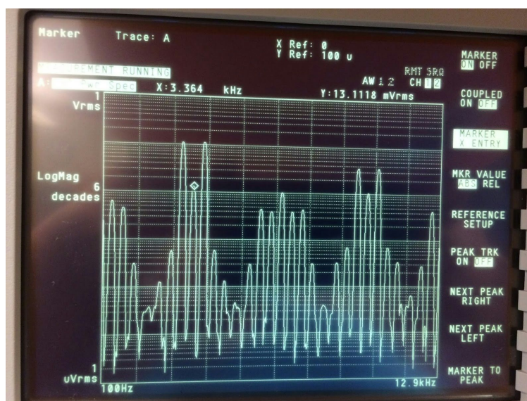
Fig. 6 Frequency content of modulator output of 400Hz with the central 3.3kHz peak
